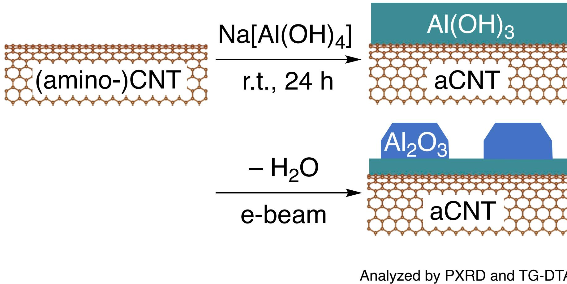
Insoluble  $\text{Al}(\text{OH})_3$  was deposited onto CNTs through hydrolysis & heterogeneous nucleation.
